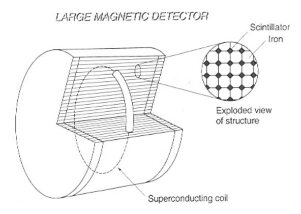
Dimension: radius 10 m, length 20 m Mass: 40 kt iron, 500 t scintillator
