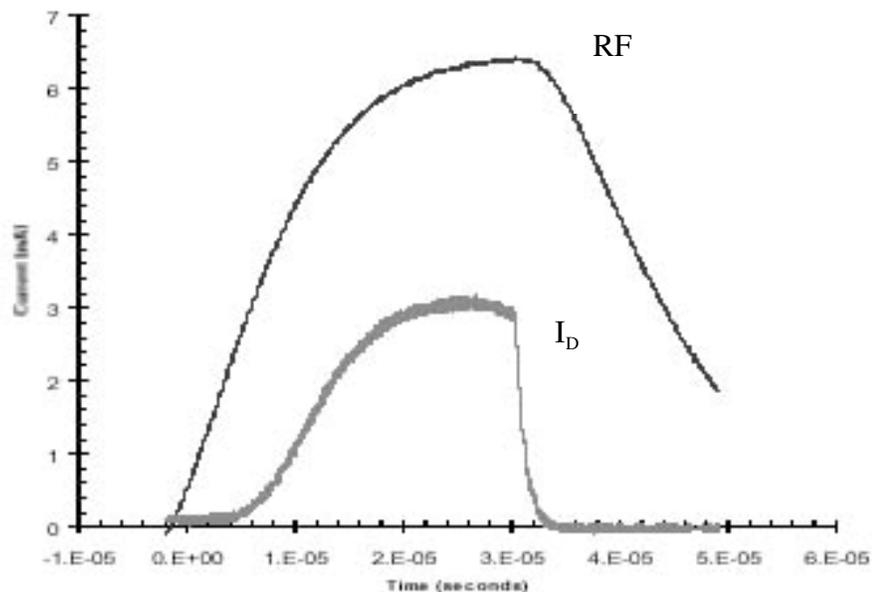
The performance of rf cavities at high power is determined primarily by field emission from cavity surfaces. This field emission creates currents which:
