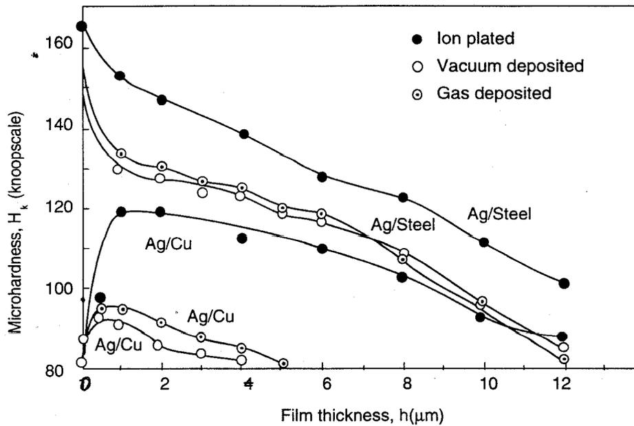
Microhardness of silver coatings as a function of film thickness deposited by three different techniques on steel and copper (data from El-Sherbiny and Salem, 1986).
