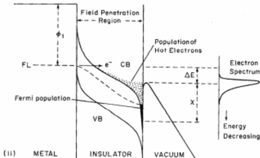
and the electrons are emitted out of the conduction band of the dielectric. The  $I$  vs  $E$  emission law is the similar, but the constants have different meanings. This process (the Richardson-Dushman law) would explain large area emission – however we seem to see local emission.
