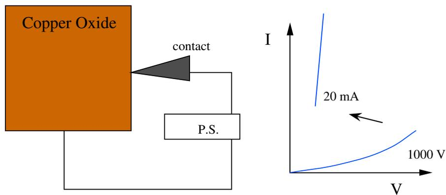
There are two resistive states here, consistent with copper filaments forming in a surface layer.
