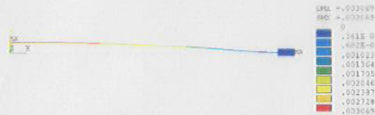
ANSYS model of buckling
