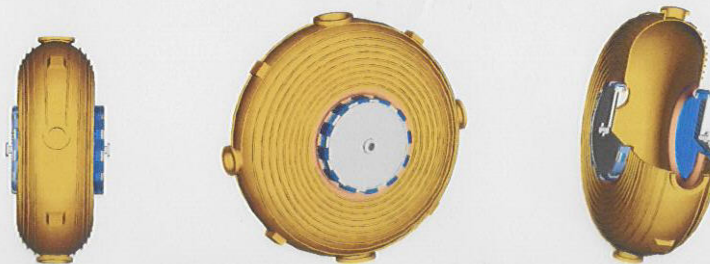
201.25 MHz cavity conceptual design
