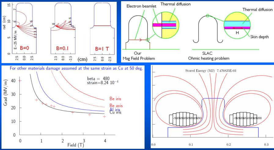
Square box cavity to study EXB effects; Be cavity to theory and RF gradient; Magnetic field shielding to avoid cavity damage by external magnetic fields
