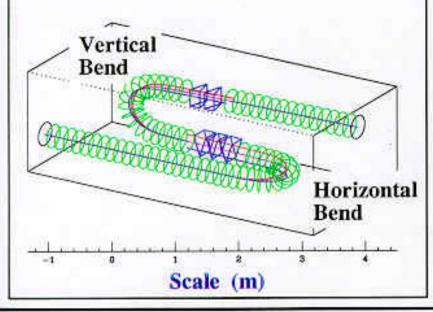
At the end of each transverse cooling stage we need a device to reduce the longitudinal emiltance
