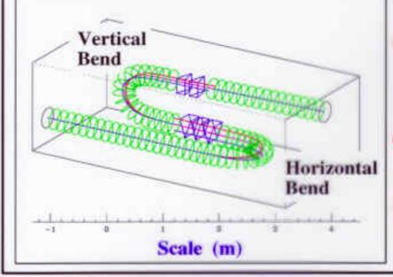
At the end of each transverse cooling stage we need a device to reduce the longitudinal emittance
