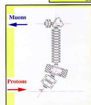
Existing low energy muon beamlines consist of a proton source, pion production target, and large aperture quadrupole decay channel with big bends to supress backgrounds.
