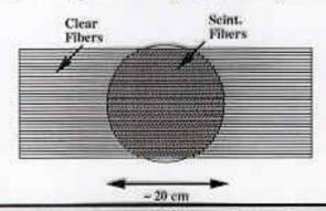
10–15 pe/MIP per fiber end 15 fiber layers Hamamatsu R5322 PMTs
