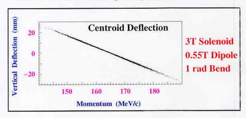
Example: To measure momentum with a precision of 0.2 MeV/c using a horizontal bend requires the vertical helix deflection to be measured with a precision of 220 μm.
