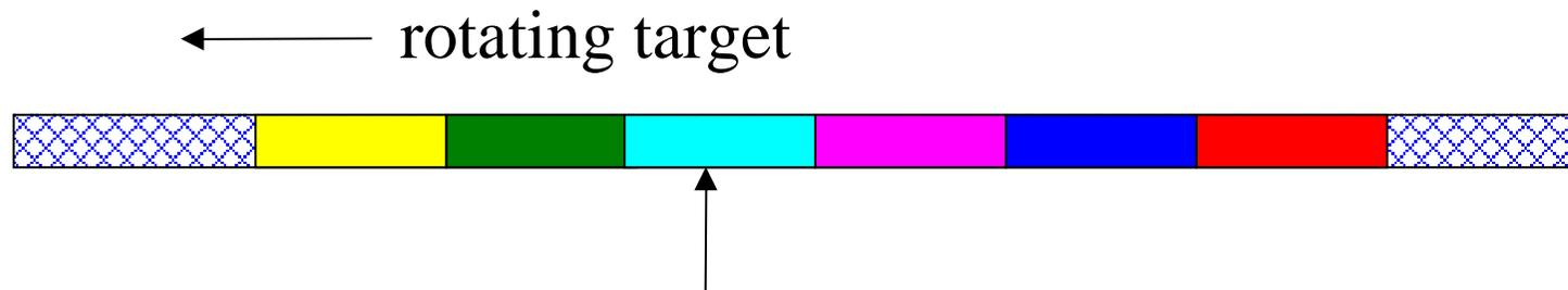
individual beam pulses on the target
