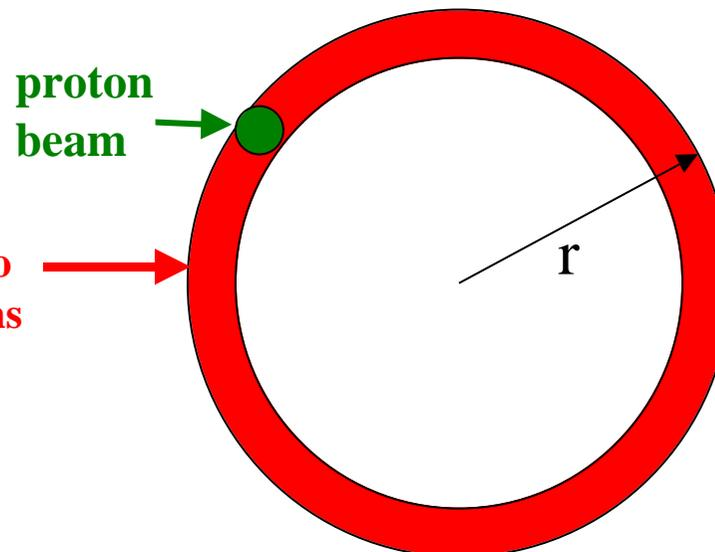
Toroid oscillates so that the beam scans the cross-section
